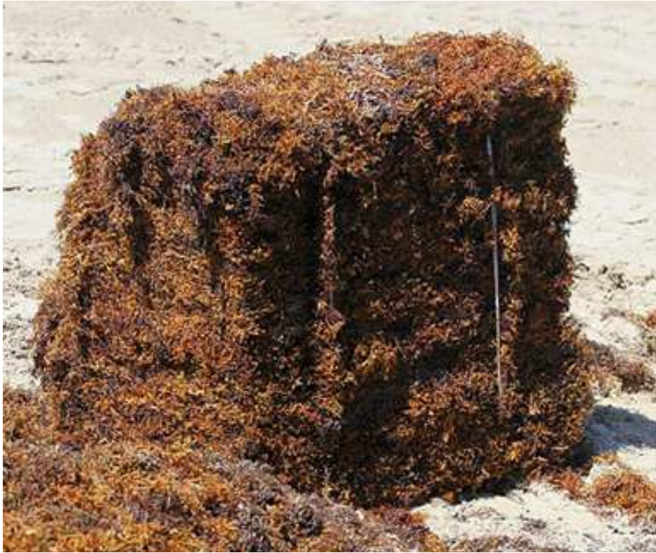
Figure 2.6: Photo of finished seabale with approximate dimensions of 2.5 \times 2.5 \times 2.0 ft. A single seabale weighs approximately 180lbs.
