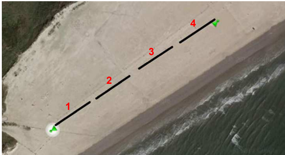
Figure 2.3: Planview of dune segment layout. The prototype dune has four segments (200 ft each).
