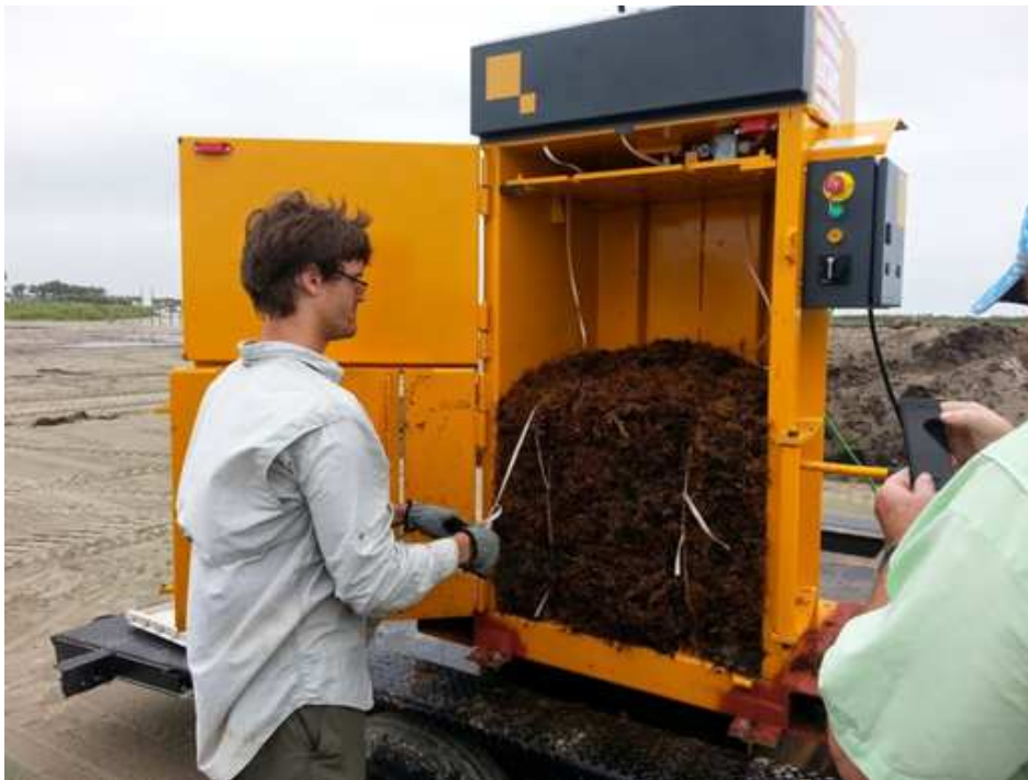
Figure 2.5: Photo of seaweed baling equipment. A vertical compactor powered by a generator was used to produce seabales for the prototype dune. The entire assembly was mounted on a flatbed trailer.
