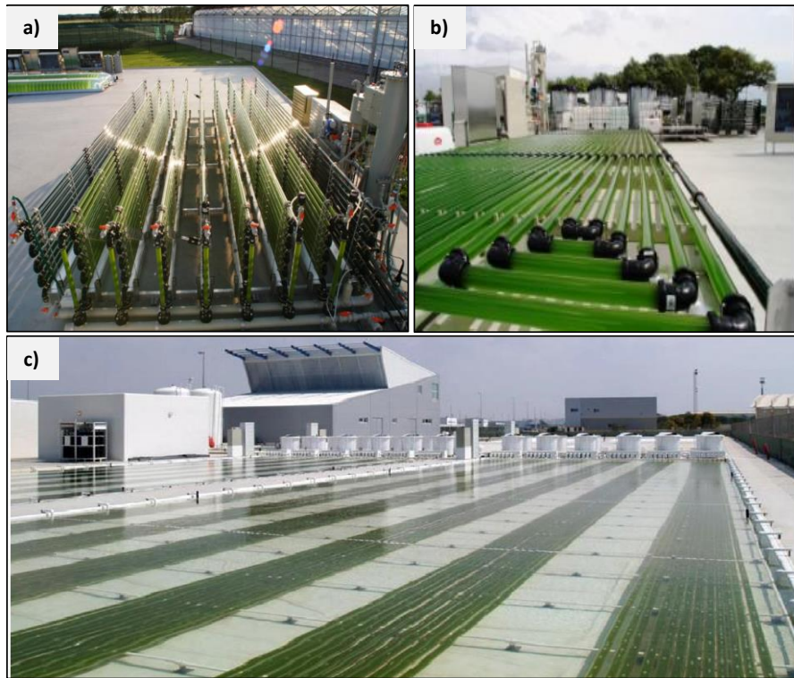
Figure 2.10. Examples of demonstration PBRs; the insets a) and b) show tubular PBR in vertical and horizontal configurations, respectively, as developed at Wageningen University (The Netherlands), from AlgaeParc website ( http://www.wageningenur.nl/en/Expertise-Services/Facilities/AlgaePARC.htm ). Inset c) shows tubular PBRs developed at Fitoplancton Marino SA (Spain), from "Miracles-specialties from algae" website ( http://miraclesproject.eu/ ).
