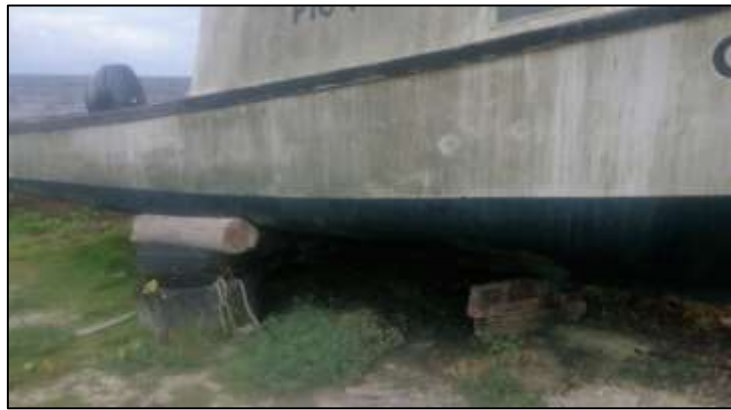
Figure 17. Black coloration on the paintwork of a ‘dry-docked’ fishing boats at Skeetes Bay, east coast, Barbados
