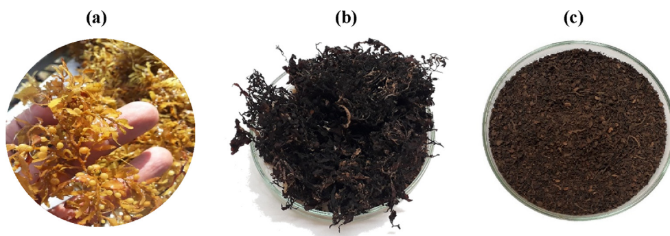
Fig. 1. Pelagic Sargassum seaweed (a) fresh from the ocean, (b) sun-dried for 2 weeks and heat treated, and (c) processed and homogenised prior to analysis.
