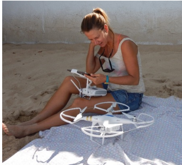
Figure 4. Author with UAS comprising UAV (DJI Phantom 3 Pro) and the GCS (remote controller and a tablet computer).
