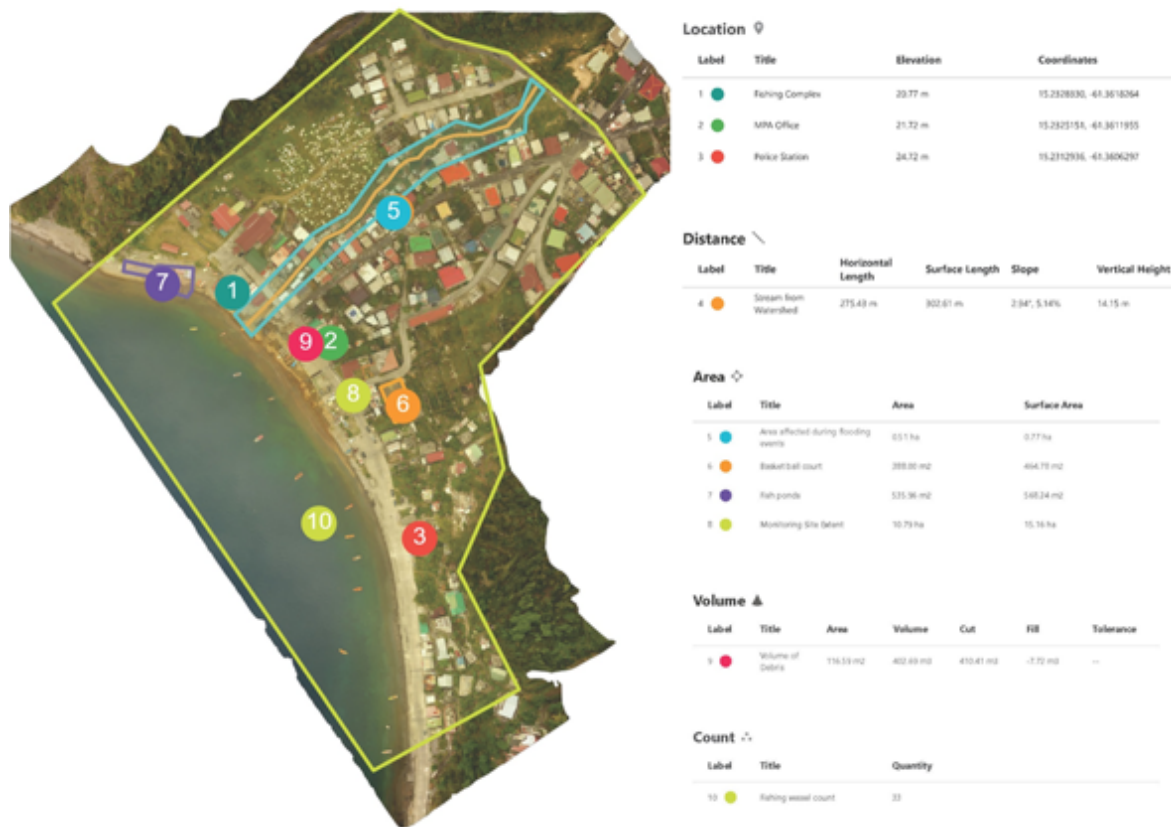
Figure 12. Example of a Drone Deploy summary report showing the drone map annotated with the location of coastal habitat and resources, fishing infrastructure and human activities that occur within the coastal community (see Appendix 3 to view full size pages).
