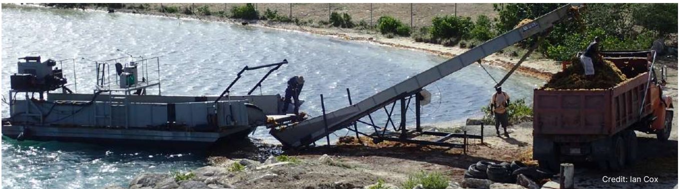
Custom conveyor belt for lifting and loading sargassum directly from boat to truck
