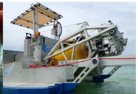
Vessel that straddles barrier for onsite repair and cleaning.
